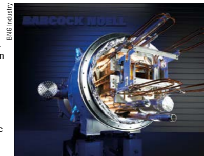
The first fast-ramped superconducting dipole for the SIS100 accelerator is currently being tested at GSI.
