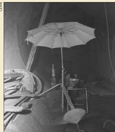
Geodetic measurements are often taken under an umbrella to shelter the surveyors from the Sun, but here a gyro-theodolite and its operator are being protected from water seeping in at the bottom of the PPI shaft, some 40 m below the surface.
